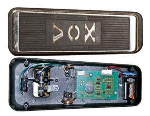
(/web/20220504054703/https://www.electrosmash.com/images/tech/v847/vox-v847-inside.png)The Vox V847 uses a single layer PCB with insertion components. The side of the board contains a Molex style connector to attach the cables to be connected to the potentiometer, footswitch and jack connectors.
